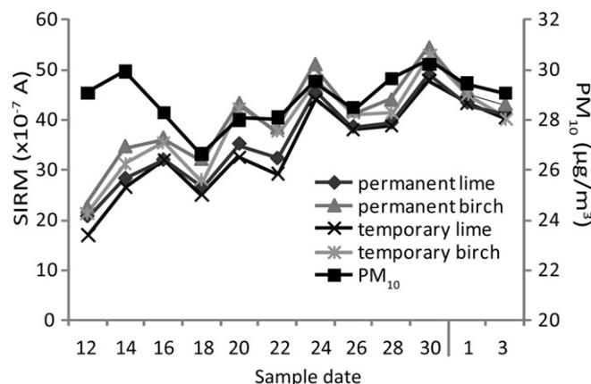
**Fig. 4.** Ambient  $PM_{10}$  concentrations (from co-located pumped-air samples) and SIRM values of birch and lime tree leaves sampled at site 2 from 10/05/08–03/06/08.
