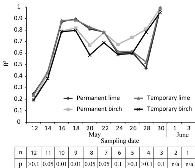
Fig. 5. Stepwise-excluded  $R^2$  values for the correlation between leaf SIRM and ambient  $PM_{10}$  concentrations. Initially, all samples were included, then stepwise removed to identify the time period after which the leaf SIRM is most reliably representative of ambient  $PM_{10}$  concentrations.
