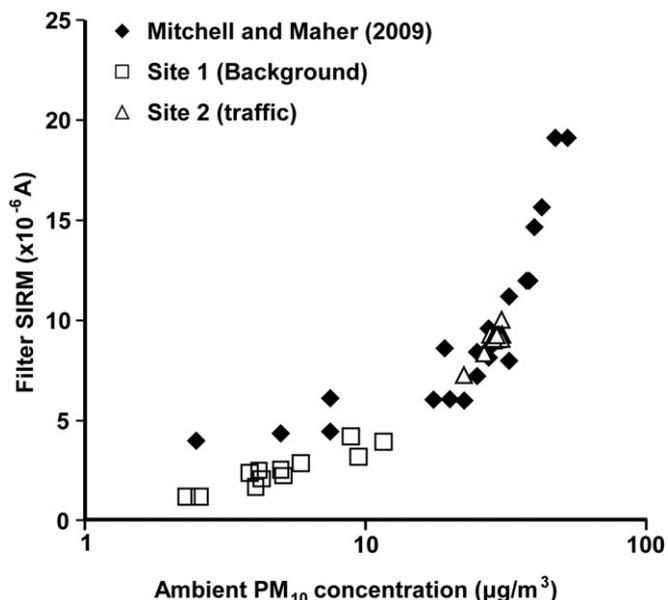
**Fig. 1.** Correlation ( $R^2 = 0.90$ ,  $n = 54$ ,  $\sigma = 0.01$ ) between filter SIRM and ambient  $PM_{10}$  concentration, sites 1 and 2 (this study) and Lancaster roadside data (Mitchell and Maher, 2009).
