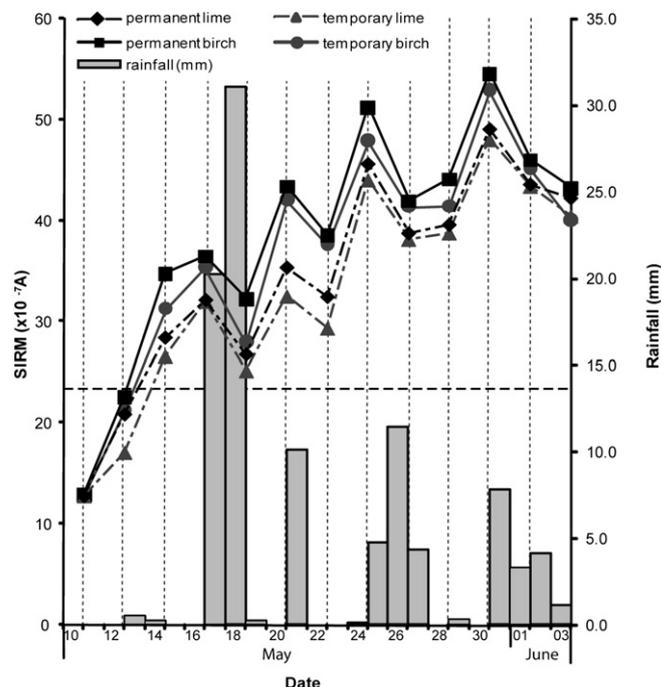
**Fig. 3.** Daily rainfall data and leaf area-normalized SIRM values of pumped-air filters and birch and lime tree leaves sampled at site 2 from 10/05/08–03/06/08. ‘Temporary’ trees were exposed only for the two peak traffic flow periods each day (08:15–10:15, 15:30–17:30).
