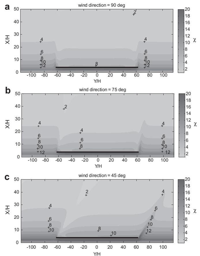
**Fig. 6.** Top view of modeled air pollutant concentrations ( $\chi$ ) at 2 m above the ground surface, for cases with a barrier of height  $H$  and incident wind directions of 90 deg (a), 75 deg (b), and 45 deg (c). The barrier is located between  $-62.5$  and  $+62.5 Y/H$  ( $750\text{ m}$  in length).
