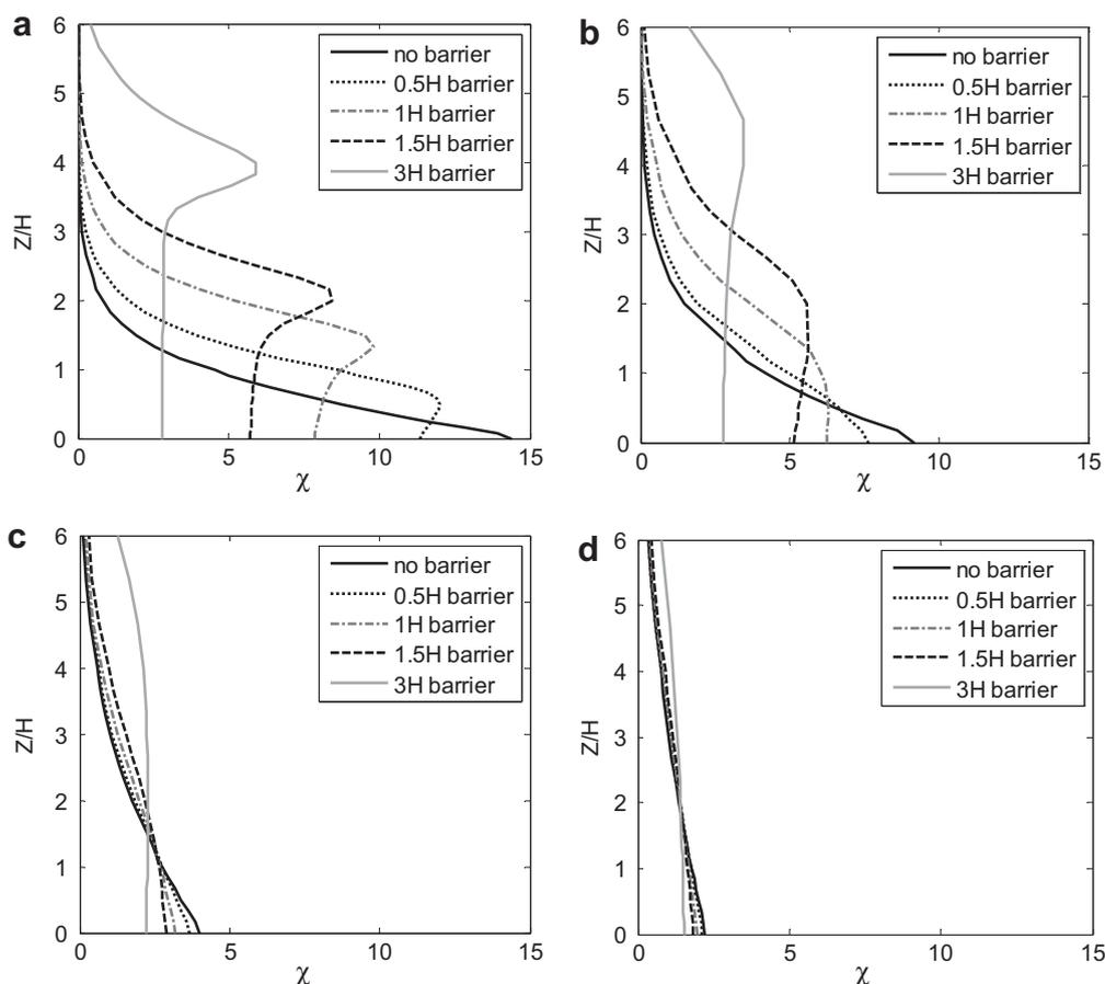
Fig. 5. Vertical distribution of normalized concentrations ( $\chi$ ) at 20 m/3.3H (a), 50 m/8.3H (b), 150 m/25H (c), and 300 m/50H (d) from the edge of the roadway under perpendicular winds, for barriers of 3–18 m compared with a no-barrier scenario. The barrier is located 9.5 m from the road edge.
