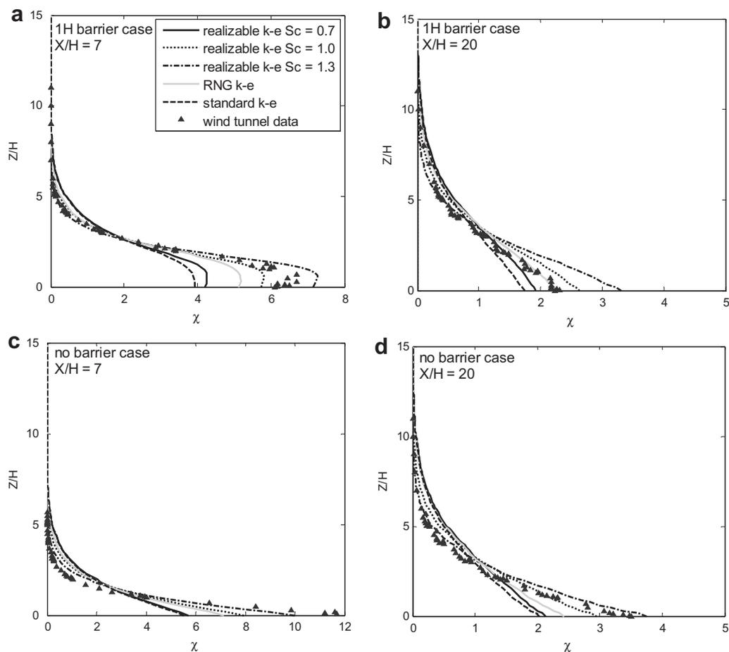
**Fig. 2.** Comparison of wind tunnel with various CFD vertical concentration profiles at different downwind distances of a road results for a barrier of  $1H$  at  $X/H = 7$  (a) and  $X/H = 20$  (b); and for a no-barrier case at  $X/H = 7$  (c), and  $X/H = 20$  (d). The center of the road is located at  $X/H = 0$ , the edge of the road is at  $2.35H$ , and the barrier position is at  $3H$  (3.9 m from the road edge).
